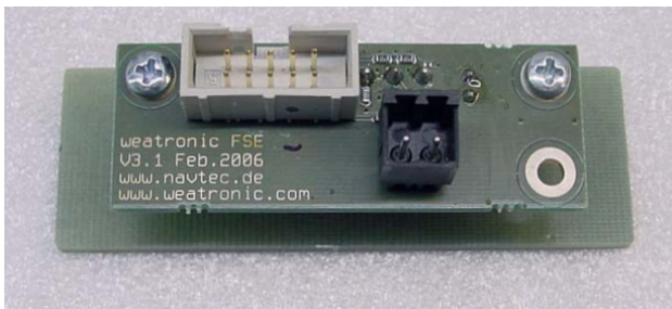
Switch board from the backside. See connector black for additional LED
